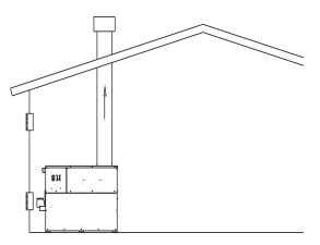
FIG. 17 Conventional Negative Draft Vertical Venting with Combustion Air Louvers
